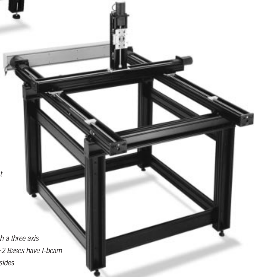
Loads bearing on the top rails are supported directly on the legs, unlike other systems that rely on fastener friction in T-slots for support
